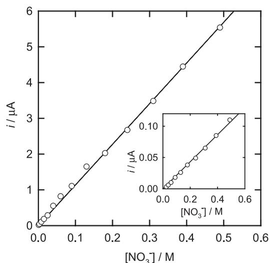
Fig. 8. Calibration curves for the reduction of nitrate at an  $H_1$ -e Rh coated  $25 \mu\text{m}$  diameter gold microelectrode (deposition charge  $90 \mu\text{C}$ ) recorded  $-1.28 \text{ V vs. SMSE}$  in  $1 \text{ M NaOH}$ . The inset shows the corresponding result for the same gold microdisc electrode coated with a plain Rh film deposited from an aqueous solution of  $\text{RhCl}_3$  in  $1 \text{ M HCl}$ .
