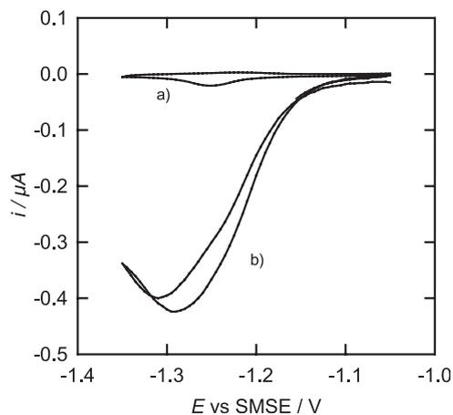
Fig. 6. Cyclic voltammograms for a  $H_1$ -e Rh coated  $25 \mu\text{m}$  gold microelectrode (deposition charge  $87 \mu\text{C}$ ) recorded at  $0.5 \text{ mV/s}$  in  $2 \text{ M NaOH}$  (a) without and (b) with  $30 \text{ mM NaNO}_3$  present.
