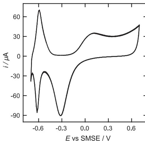
Fig. 5. Cyclic voltammogram of an  $H_1-e$  Rh film (126 nm thick, total deposition charge  $3.5\text{ mC}$ ) deposited from the  $C_{16}EO_8$  template mixture on a gold disc electrode (area  $0.0079\text{ cm}^2$ ) recorded at  $50\text{ mV/s}$  in 1 M sulfuric acid. The film was soaked in water for 1 h prior to the measurement.
