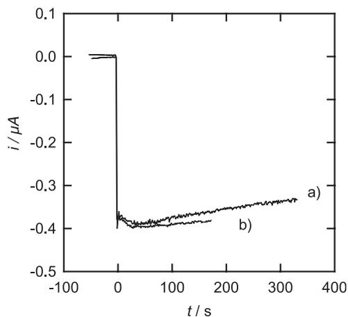
Fig. 7. Transient responses for an  $H_1$ -e Rh coated  $25 \mu\text{m}$  diameter electrode following addition of  $50 \text{ mM}$  nitrate to  $2 \text{ M NaOH}$  recorded at  $-1.28 \text{ V vs. SMSE}$ . The  $H_1$ -e Rh film was deposited onto the gold microelectrode surface from the template mixture using a deposition charge of  $90 \mu\text{C}$  corresponding to a film thickness of  $126 \text{ nm}$ . Curves (a) and (b) show results for replicate measurements in fresh NaOH solution.
