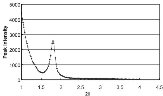
Fig. 3. Low angle X-ray diffraction of an  $H_1-e$  Rh film deposited on an evaporated gold electrode from a mixture of 12 wt.%  $RhCl_3$ , 47 wt.%  $C_{16}EO_8$ , 39 wt.% water and 2 wt.% heptane. The total charge passed for deposition was  $0.70\text{ C/cm}^2$ .
